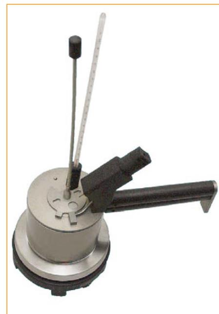
Figure 1: Drew Marine Flash Point Test Kit
