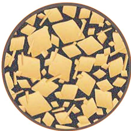
Figure 3: Broad microcrystalline wax formation of untreated fuel
