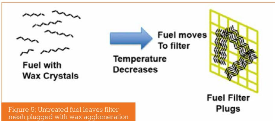
Figure 5: Untreated fuel leaves filter mesh plugged with wax agglomeration
