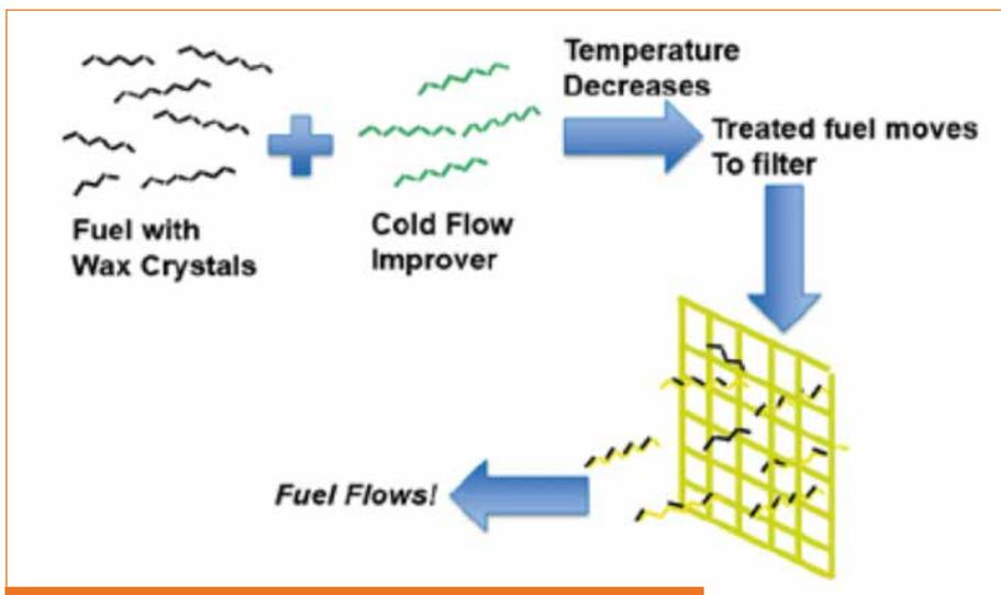
Figure 6: After being properly treated with cold flow improver, fuel flows without agglomerating on filter mesh
