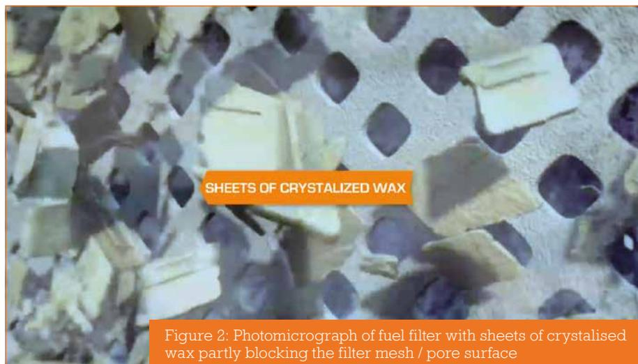
Figure 2: Photomicrograph of fuel filter with sheets of crystallised wax partly blocking the filter mesh / pore surface
