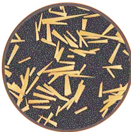
Figure 4: Narrow microcrystalline wax formation of fuel treated with cold flow improver
